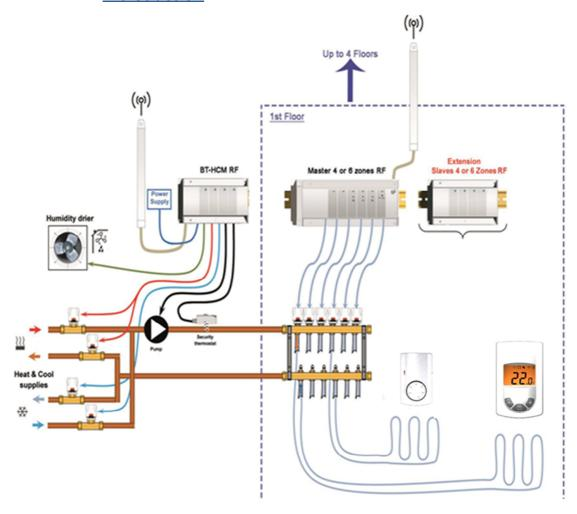
The thermostat is able to communicate with the current products (unidirectional wireless communication "rF.u") and with the products of the new range (bidirectional wireless communication "rF.b").
