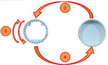
> Step 5: replace central button (do not turn button during this operation)
